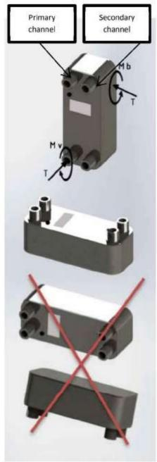
BPHE mounting position must ensure sufficient space around the unit to be able to carry out maintenance works and service. Installation position must allow the possibility of venting and drainage.
